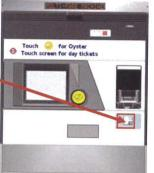
The card reader is now flush to the front of the device, hopefully making it a lot more difficult to attach a skimming device and conspicuous if anyone does try to.
