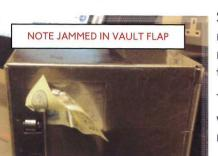
Subsequent investigation by Cubic, based on some observations by a number of staff, that the problem was potentially linked to the way that the note was inserted into the device by the customer, have now established the cause of this issue.
