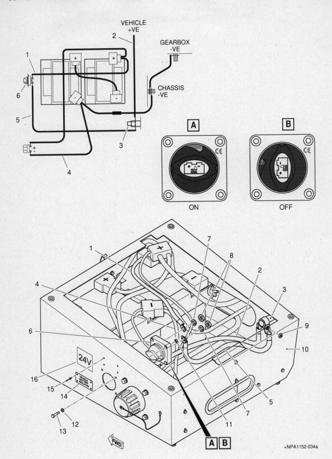
Fig 11 VEHICLE BATTERY ISOLATOR switch installation
