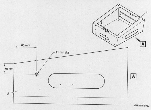
1 LH seat base 2 LH inboard side
