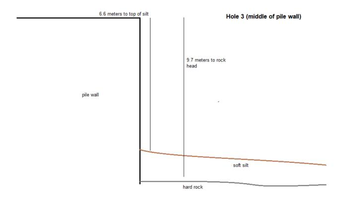
The diver reported that the material removed from in front of the pile wall was soft silt that was easily removable with the airlift. The diver followed the pile down 3.1 meters into the silt and reported that he had found the rock head. It appeared to the diver that the pile entered the rock head and continued, however, the diver could not inform on how much embedment the pile may have into the rock.
