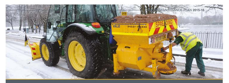
Gritter bodies have been changed from diesel to hydraulically powered units, which when considered with the reduction in vehicles within the gritting fleet has resulted in a significant reduction of CO2 emissions.
