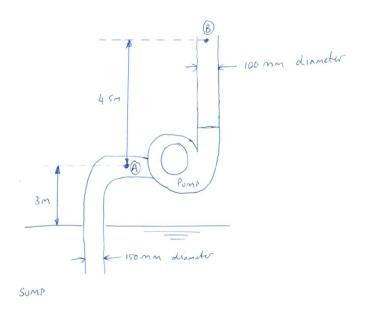
i) Determine the pressure at A and B neglecting all losses from the system.
