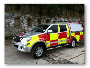
Toyota Hilux – 3.0 Litre with a Briggs & Stratton Vanguard petrol engine driving a Hale HPX 75 pump
