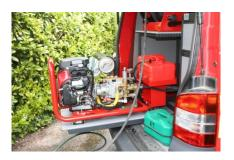
**Option 2** VW T5 3.2T Van with a Vehicle Misting Systems Pump driven by a 6.5HP Briggs & Stratton Vanguard pump
