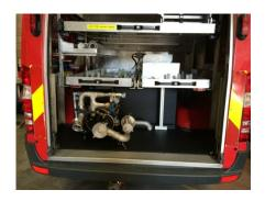
**Option 5** Mercedes Sprinter (LWB) 5.3T van with a Briggs and Stratton petrol engine driving a Hale HPX 75 Pump
