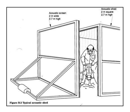
Simple Acoustic Enclosure for Stationary Plant –suitable for any plant. Advantages: Best Level of Noise Reduction, simple, quick to erect, demountable, re-usable.
