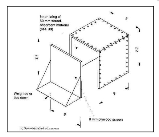
Open-Sided Shed with Baffle – suitable for any plant (i.e. generators, kango breakers). Advantages: Improved noise reduction, simple, quick to erect, demountable, re-usable and easily movable for platform works.
