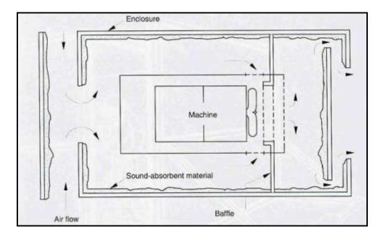
Simple Acoustic Enclosure for Stationary Plant –suitable for any plant. Advantages: Best Level of Noise Reduction, simple, re-usable.
