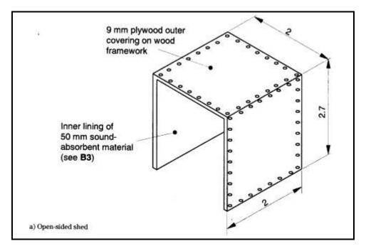
Open-Sided Shed – suitable for any plant. Advantages: Simple, quick to erect, demountable, re-usable.
