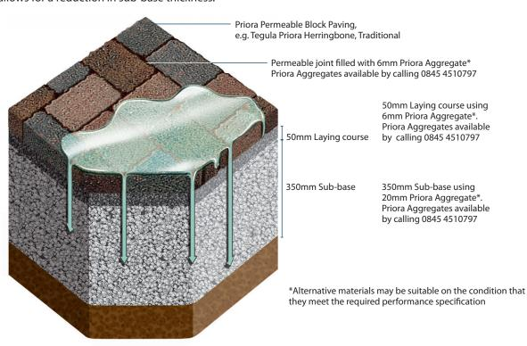
This example uses Tegula Priora Herringbone, Traditional. All Priora products which can be laid in the Herringbone laying pattern are suitable for this application. For advice on laying patterns by application, please contact the Water Management Design Team: 0845 30 20 606
