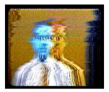
**Background:** If you are watching analogue television, this is a common symptom of a weak signal. This may be due to a transmitter fault or a problem with your own installation.
