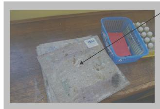
G.P. Area – heat pads are an ACM (sample BS/08). Although they are in good condition, it is recommended they be replaced with a non asbestos material.
