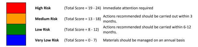
The risk assessment scores detailed within this report should be used as a means of prioritising work. The recommendation given is largely based on reducing the material assessment parameters, e.g. through encapsulation or removal. When deciding on prioritisation and the required action, full consideration should also be given to controlling the priority assessment parameters, e.g. through restricting access etc.
