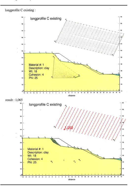
The slope safety factor of the existing slope is 1.06 very near to 1. The bad thing is that there is almost a permanent risk of a slope sliding in the upper part of the slope but the impact will be moderate due to the un-profound depth of the slip surface. Only the fence of the side would be probably impacted.
