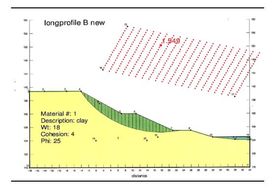
Finally the safety factor of the original same slip surface increase from 1.25 to 1.55 or an increase of 20%.
