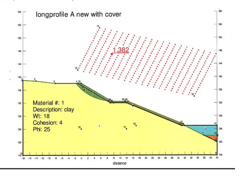
The anti-erosion structure (Geocells) has a computed slope factor of safety of 1.38 or another increase of  $10\,\%$  on the re-profiled slope. The factor of safety generated by utilising MacMat-R is about 1.34 or a 5% increase on the Option A.
