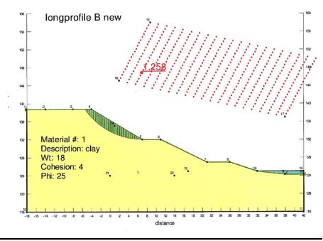
The new slope safety factor of 1.26 is almost unchanged but the volume of the slip area is far reduced and is only situated at the top part of the slope. If a collapse would happen only a small un-deep part of the upper slope would be impacted and the damage to the capping would be limited. To have an
