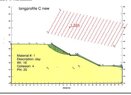
The anti-erosion structures (Geocells) have now a computed slope factor of safety of 1.33 or an additional increase of 10 % on the re-profiled slope. The factor of safety for utilising MacMat-R is about 1.28 or a 5% increase on Option A.
