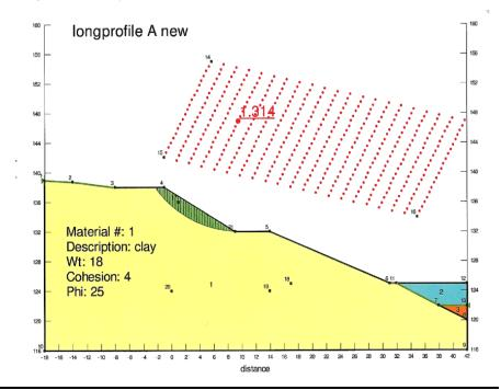
The re-profiled slope has now a slope safety factor of 1.3 instead of 1.1 this means an increase of 20 % in the slope stability.
