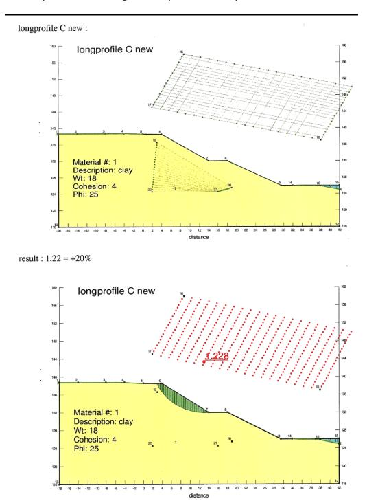
The re-profiled slope has now a slope safety factor of 1.22 instead of 1.06 this means an increase of 20 % in the slope stability.
