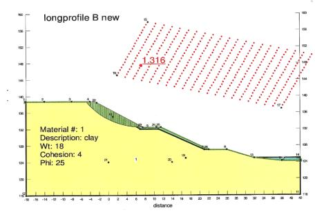
The anti-erosion structures (Geocells) have a computed slope factor of safety of 1.32 or another increase of 5% on the re-profiled slope. The factor of safety for utilising MacMat-R is about 1.29 or a 2.5 % increase on Option A.
