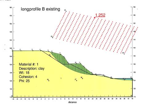
The slope stability factor on the existing slope profile is 1.25 but when the slope is slipping the total soil movable mass is large due to the quite deep slip surface. The bigger the shaded green area the bigger the impact of the slope
