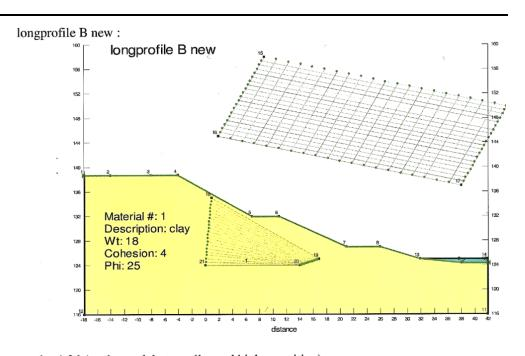
result: 1,26 (unchanged, but smaller and higher position) global stability of the same slipzone as existing: 1,55 (see next page) thus here also an important gain in stability.
