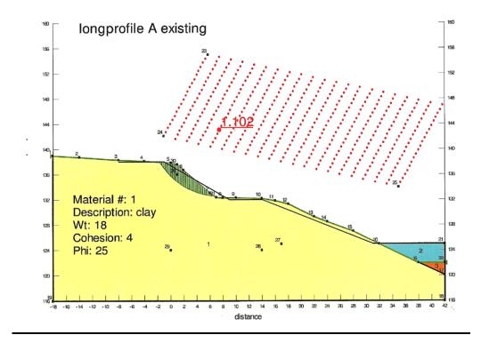
For the existing slope we have we have an estimated slope safety factor of 1.1
