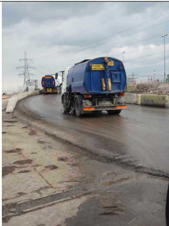
Two of several road sweepers we have on site that manage the hard-surfaced haul routes
